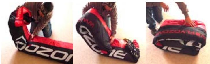
**IMPORTANT: Do NOT lay the wing flat on the ground before packing the glider, this will cause abrasion damage to the top surface as you pull the glider towards the middle. ALWAYS pack from a mushroom or lift the wing off the ground when gathering the wing and grouping the leading edge.**
