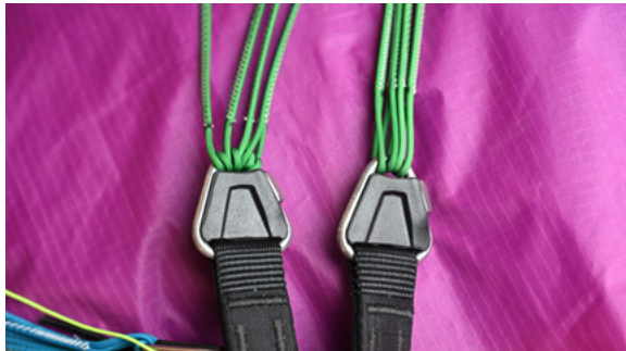
Left : loops on the maillons; right: loops released
