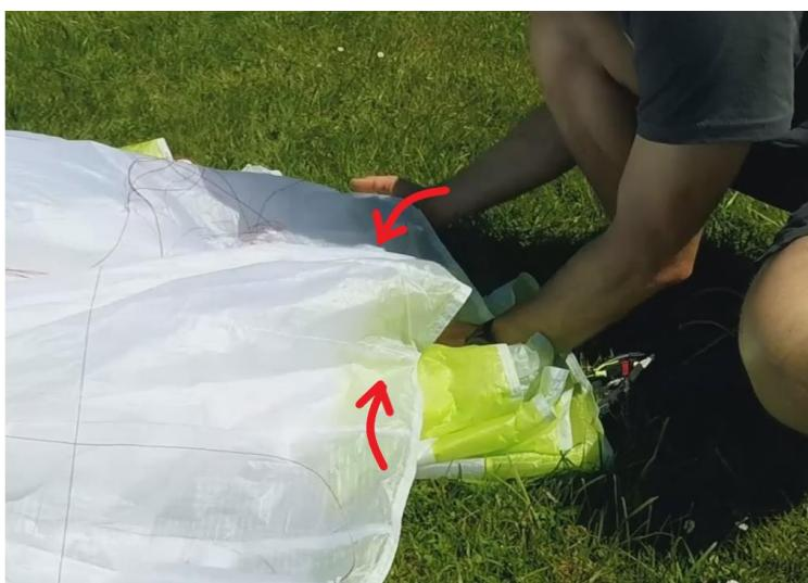
6. Using the **AirPack 50/50**: Fold the wing up from the trailing edge one time at the length of the innerbag.
