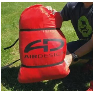
By using the standard „**AirPack**“, the whole glider will be put into the inner-bag first, then closed, and then folded to the required length and fixed with the straps.
