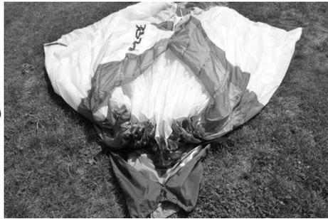
3. Lay the leading edge flat on the packing bag / AirPack and secure with the strap just below the end of the polyamide rods.
