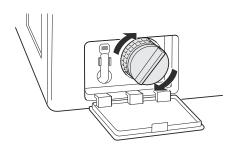
Close the drain pump filter cover.
