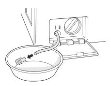
4 Remove the pump filter.
