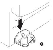
2 Fit the hinge ② over the hinge lever latch ③ and slot it into place. Rotate the lever ④ clockwise and fasten the hinge.
