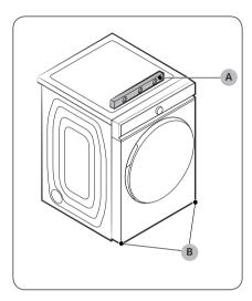
Using a **level (A)**, check if the dryer is level side to side and then front to back. If the dryer is not level, turn the **leveling feet (B)** clockwise to lower the dryer or counterclockwise to raise the dryer.
