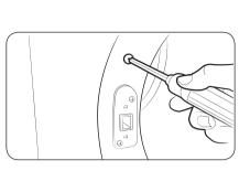
6. Remove the two screws above and below the lever holder on the opposite side of the door opening.
