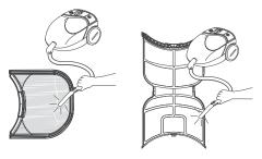
If the lint filter has become very dirty or clogged with fabric softener, wash the lint filter in warm, soapy water and allow it to dry thoroughly before reinstalling.
