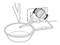
Clean the pump filter and opening.
