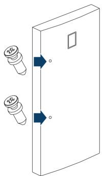
**3** Loosen the hex screws on top and bottom of the handle with the hex wrench (provided) so that you can fit the handle over the extended head screws in the door.
