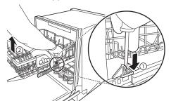
**3** To remove the back rack supports from the rails, hold a side rail with one hand, lift the front of the rack, and firmly push the rack
