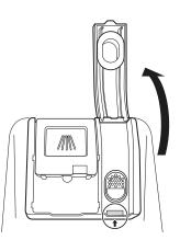
2 Add a liquid rinse aid to the maximum fill level. Allow the rinse aid to settle in the dispenser while filling, or air bubbles may result in poor drying performance. Avoid overfilling the dispenser.
