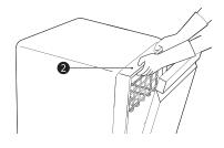
1 Align the dishwasher with the opening. Make sure the water supply line and electrical cable are in the correct positions to slide into their channels properly.
