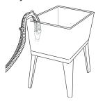
Use the provided tie strap to secure the drain hose in place.
