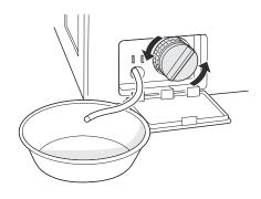
**5** Clean the pump filter and opening.
