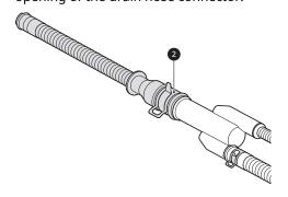
4 Securely connect the short drain hose to a floor drain or standpipe.
