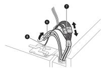
3 Rotate the hinge lever **9** counterclockwise. Lift the top hinge **10** free of the hinge lever latch **①**.
