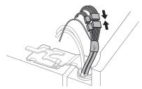
**4** Push the water supply lines into the hole on the top case and pull them through the backplate.
