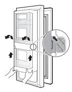
**2** Pull out the crisper to full extension, lift the front up, and pull straight out.
