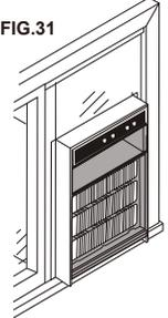
**37** Drill two 9/64" diameter pilot holes in the top window jamb in line with the partially plugged holes in the panel frame. Secure the panel frame to the window jamb with two #8-32 x 3/4" self-threading screws. If additional holding is necessary, two screws may be used on the sides of the panel frame as well.
