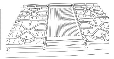
Replace the center grate with the reversible cast iron griddle
