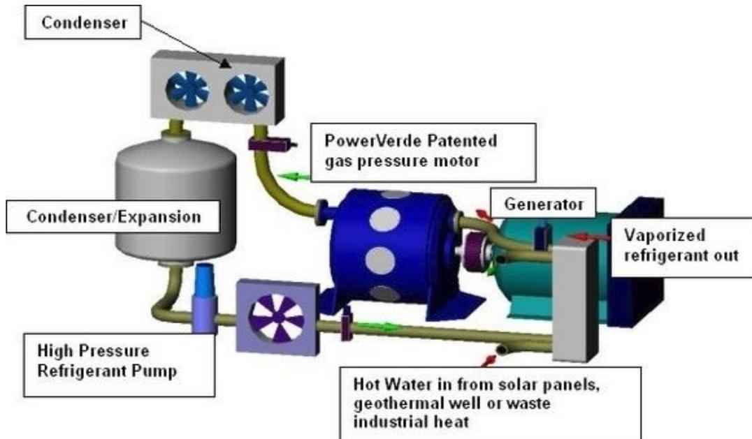
Waste Heat recovery captures heat from an existing industrial process, examples include:
