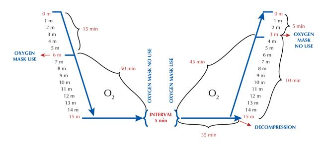
Figure 2 - Diagram illustrating the pressure (atmospheres absolute) and time of the hyperbaric chamber.
