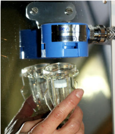
1. Detach the adapter sight glass and place Bevi Tab flat
