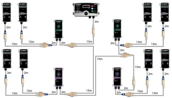
1 x Central Display; 2 x CO<sub>2</sub> Sensors; 2 x O<sub>2</sub> Sensors; 8 x Alarms
