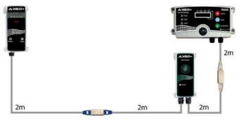
1 x Central Display; 1 x CO<sub>2</sub> Sensor; 1 x Alarm
