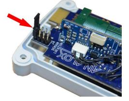
The image to the left shows the jumper link at location 1 (Factory default). Each Sensor PCB contains a SENSOR
