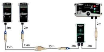
1 x Central Display; 1 x CO<sub>2</sub> Sensor; 2 x Alarms
