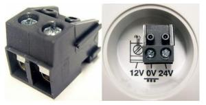
(left) The beacon terminal block. Ensure this is fitted on the 0 V and 24 V terminals (right)
