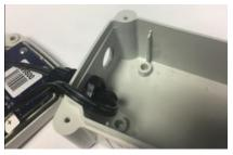
[4] Fit a gland blanking disc over the hole which the gland and cable were removed from.
