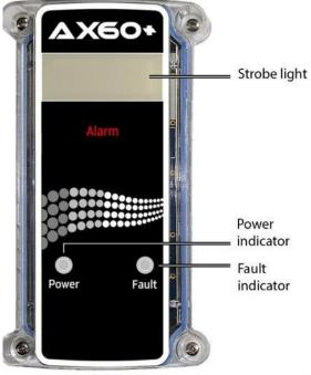
NOTE: The sounder is on the rear of the enclosure
