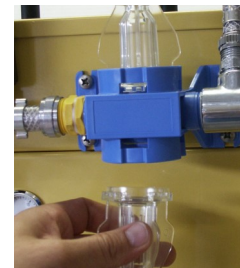
6. Fasten the adapter sight glass at the valve again
