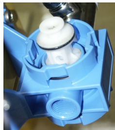
4. Lubricate the O-ring with grease for valves, and place the piston with the bore holes side-by-side towards the water intake side
