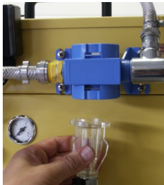
1. Detach the adapter sight glass from the valve
