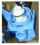
4. Lubricate the Oring with grease for cocks, and place the piston with the bore holes side-by-side towards the water intake side
