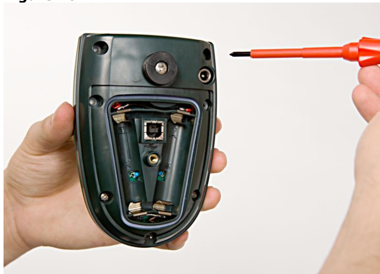
Figure 16 Remove the sensor cap screws
