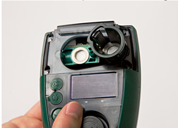
Figure 20 Correct extraction tool position
