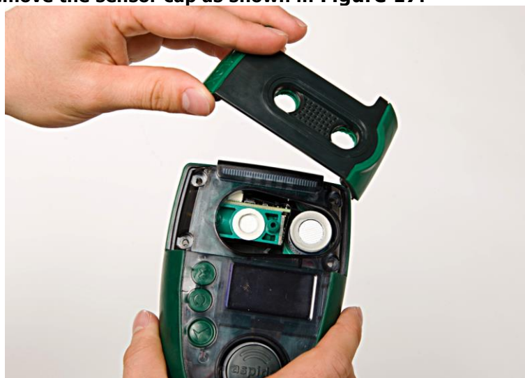
Figure 17 Remove the sensor cap
