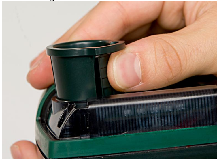
Figure 21 Squeeze the extraction tool
