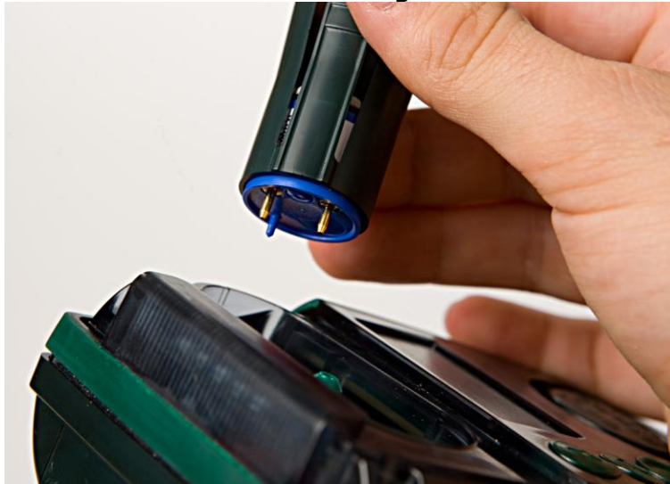
Figure 22 Removing the oxygen sensor
