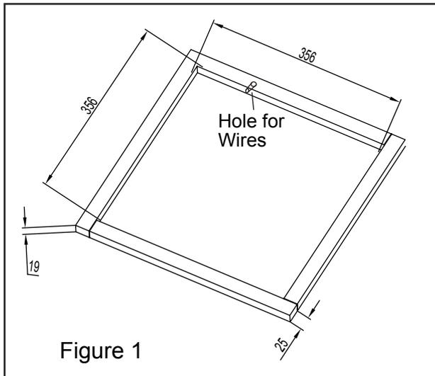
1. It must be capable of supporting both the weight of the roof top air conditioner and the interior ceiling assembly.
