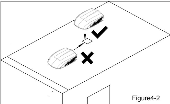
2. Fix the outdoor unit at the roof of vehicle and then drill holes.
