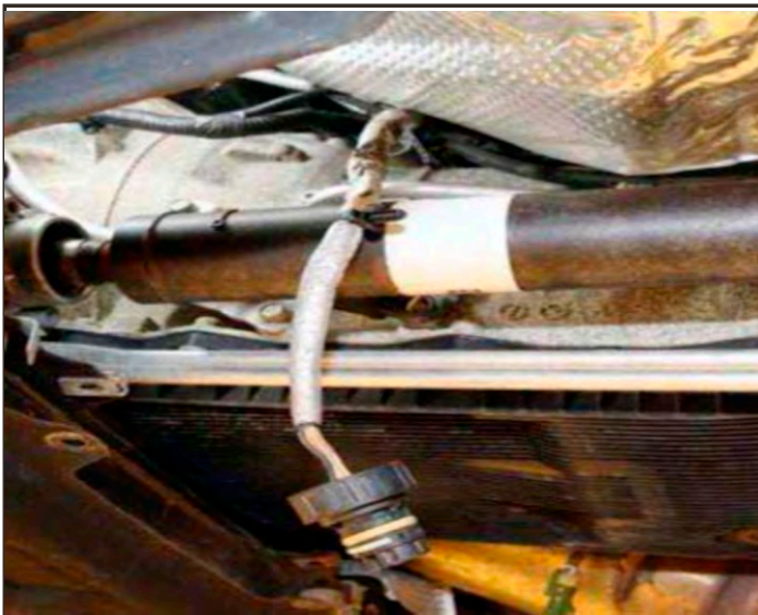
Swing Wire Harness To Left Side Of Vehicle For Access.
