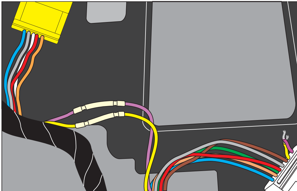
The GMLAN Communication Wires Were Cut From The VCIM And Spliced Together
