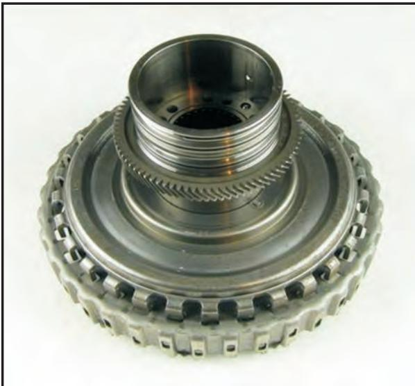
8. As the distributor sleeve is placed onto the clutch housing with the notches aligned, the notch in the distributor sleeve should also be aligned with the pressure feed slot in the clutch housing.
