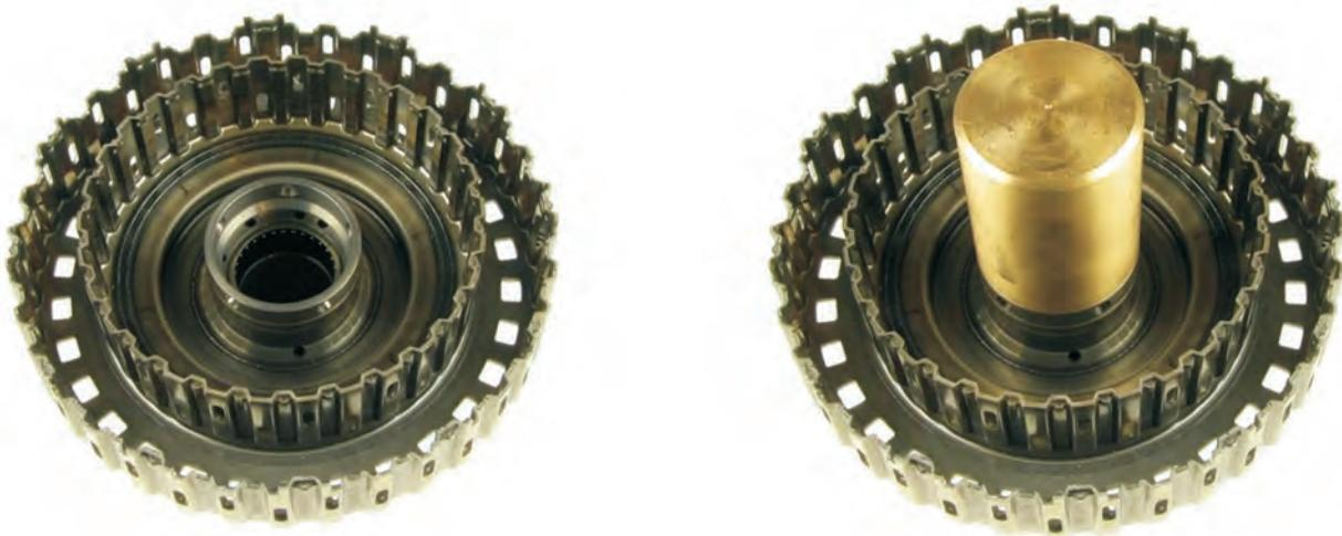
1. Install a support plug into the open face side of the double clutch housing as shown above.
