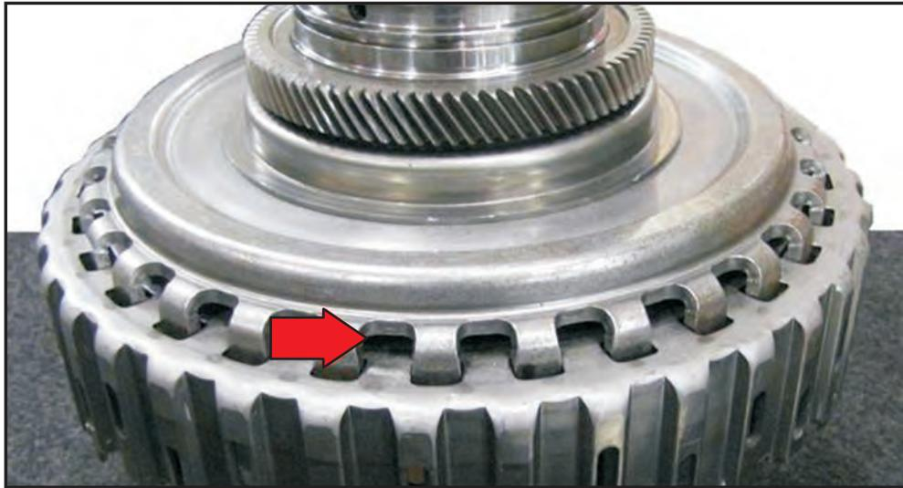
24. With the distributor sleeve in place, use a small amount of air to check the K1 piston for proper movement.
