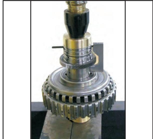
13. Once the sleeve is down by approx. 6.35mm (.250"), remove the tool.
