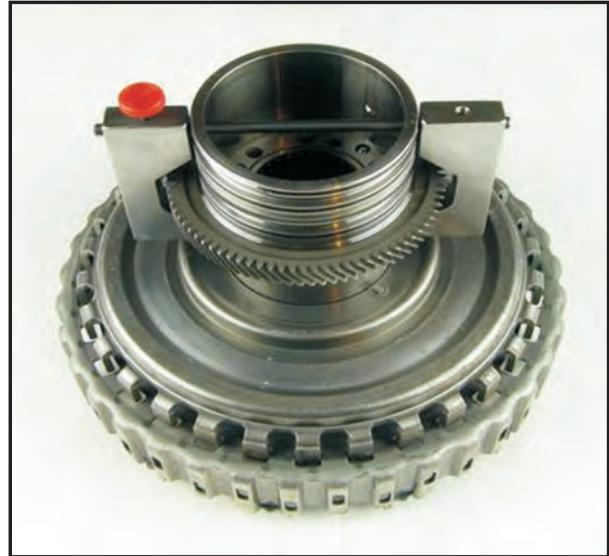
9. Secure the alignment position with a suitable alignment tool such as the one designed by ALTO. It aligns the K1 and K2 clutch feed holes in the sleeve to the clutch housing. The jaw tool fits into the K1 feed slots in the drum assisting in the alignment process.
