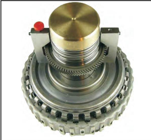
10. Install the slotted press plug over the alignment tool.
