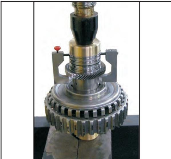
12. As the sleeve begins to be pressed onto the housing, open the jaws of the alignment tool.
