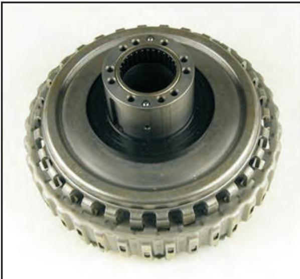
4. Align the apply fingers of the K1 clutch piston to the access holes in the clutch housing and install the piston.
