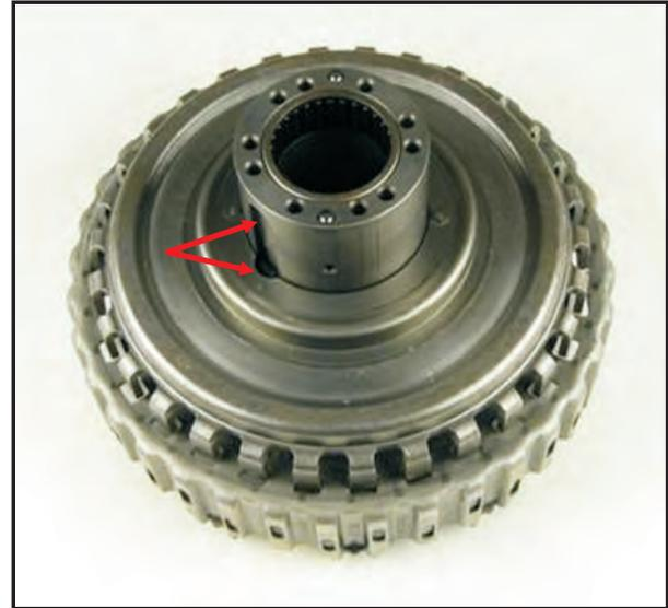
5. Install the piston seal cap with the notch aligned to the pressure feed slot in the clutch housing.
