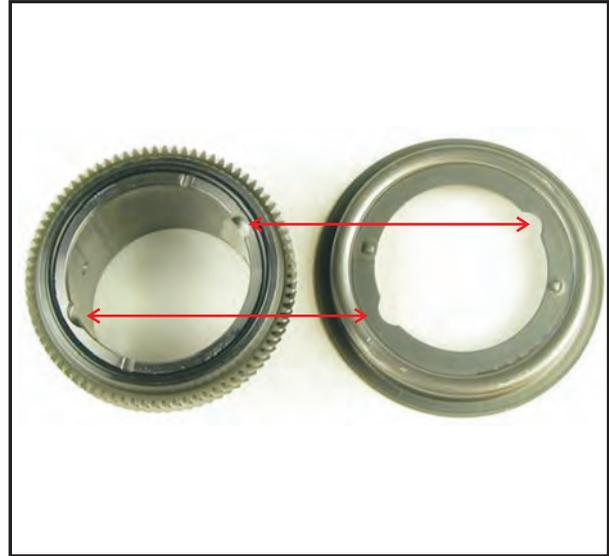
7. Align the notches in the distributor sleeve to the notch in the piston cap.
