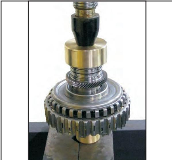
20. With the tool removed, carefully press the sleeve to the housing.
