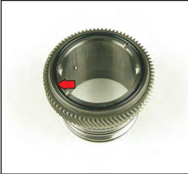
6. Install the o-ring into the distributor sleeve in the location shown above.
