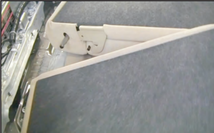
To gain access to the hybrid battery/inverter, the rear seat backs will have to be disconnected from their pivot points.
