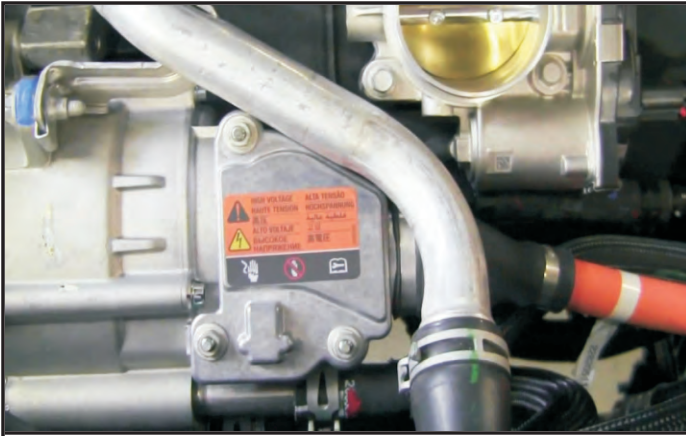
One of Two high voltage interlocks is located on the BAS assembly with the appropriate warning label.
