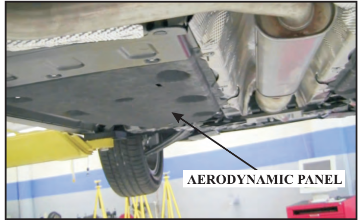
The underside of the vehicle has numerous panels bolted to the body for aero-dynamic purposes.
