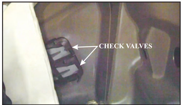
The hybrid battery cooling system duct work ends in the driver side rear wheel well. Built into the body are check valves that let used air out but lets nothing into the vehicle.
