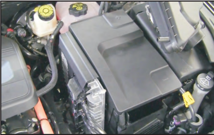
The 12 Volt battery is located in the engine bay on the driver side. Disconnect the cables if working on high voltage circuits.
