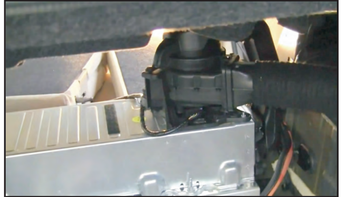
The Hybrid battery box is electrically air cooled by a 12 Volt fan and a complex duct work system which brings in fresh air and exhausts the exiting air out of the vehicle.
