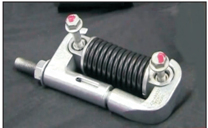
When disconnecting the BAS belt tensioner damper spring, use Kent-Moore Tool #EN-48932 or similar device to avoid injury.
