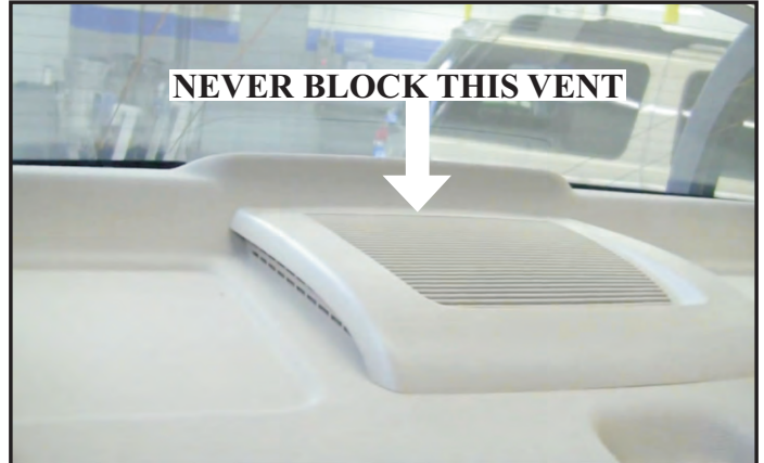
Fresh air to cool the hybrid battery pack is drawn in through the vent located on the rear package shelf.
