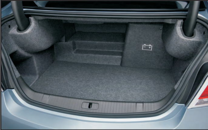
The Lithium Ion Battery Pack is located under a cover. Access to the cover is through the trunk.
