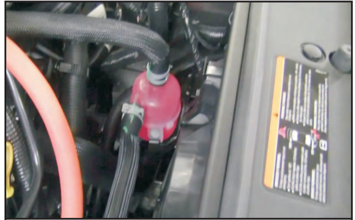
Mounted on the driver side inner fender is the 12 Volt dedicated BAS coolant pump.
