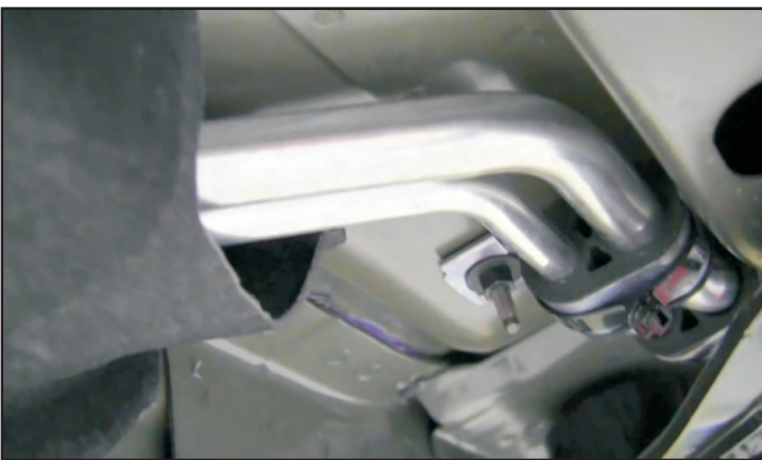
Electrical conduit carries the high voltage cables from the battery box in the rear of the vehicle to the BAS assembly in the front of the vehicle. The conduit is exposed only in a few areas as most of it is concealed behind the under body aero-dynamic panels.
