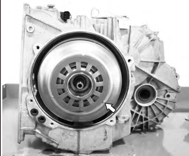
Remove B and E Clutch housing
