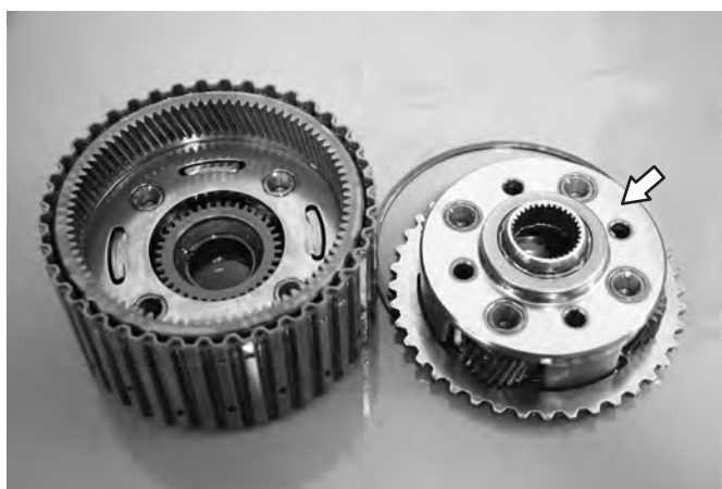
Remove Planetary
