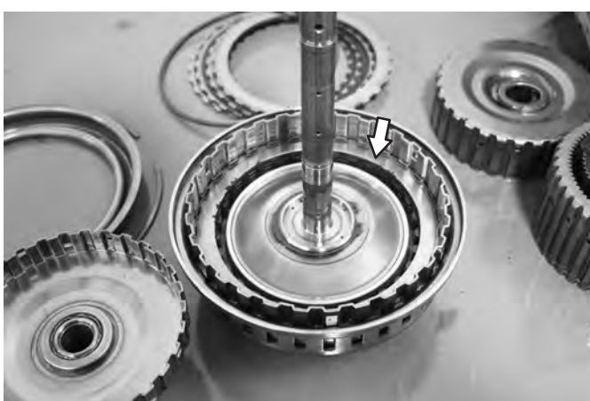
Remove E Clutch
