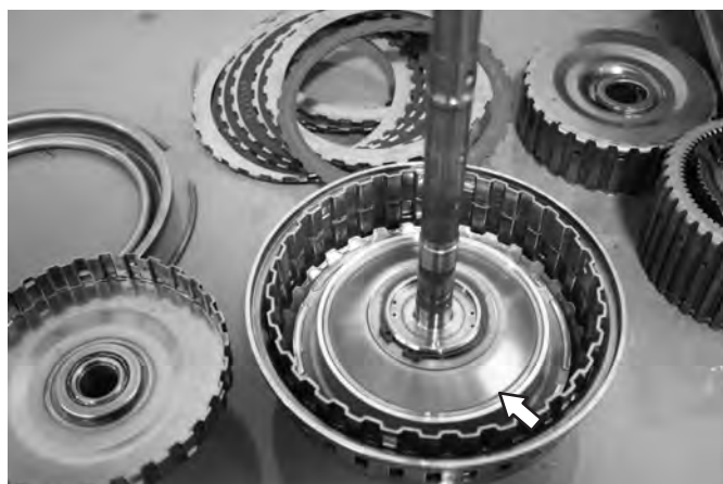
E Clutch apply piston
