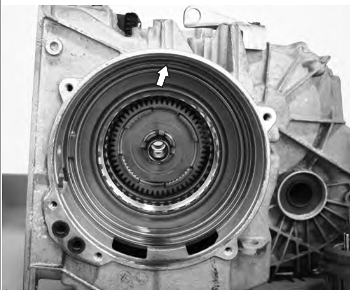
Remove snap ring for C Brake
