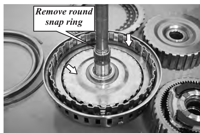
Remove snap ring and E Clutch hub
