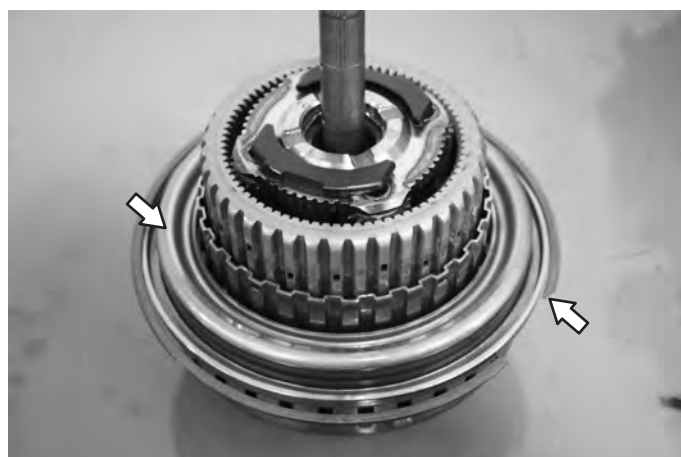
Remove snap ring and B Clutch apply cup
