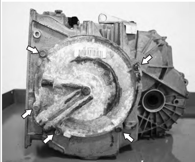
Remove the rear cover retaining bolts and cover
