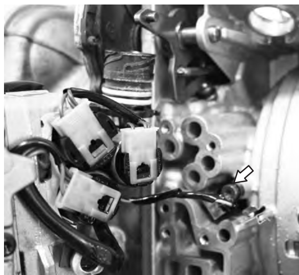
Remove Valve body. remove 27 torx OSS retaining bolt and remove the sensor- note there is a .099" shim in between the sensor and the case
