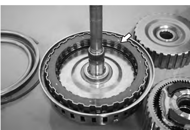
Remove B Clutch
