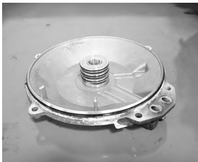
B and E Clutch Sealing rings
