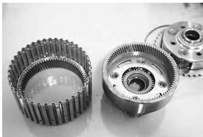
Remove lower planetary
