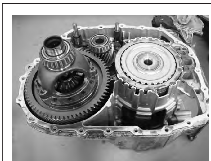
Remove Bellhousing Differential
