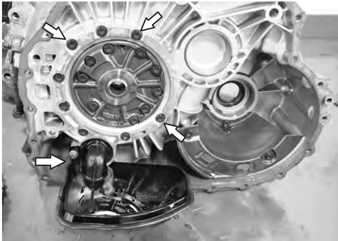
Remove 10mm filter attaching bolt and filter Remove 27 torx pump to case bolts
