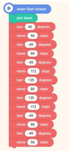
To start drawing the figure shown, place your character in the position X = 0 and Y = 0, keep in mind that the turns of this figure are made at 45° angles
