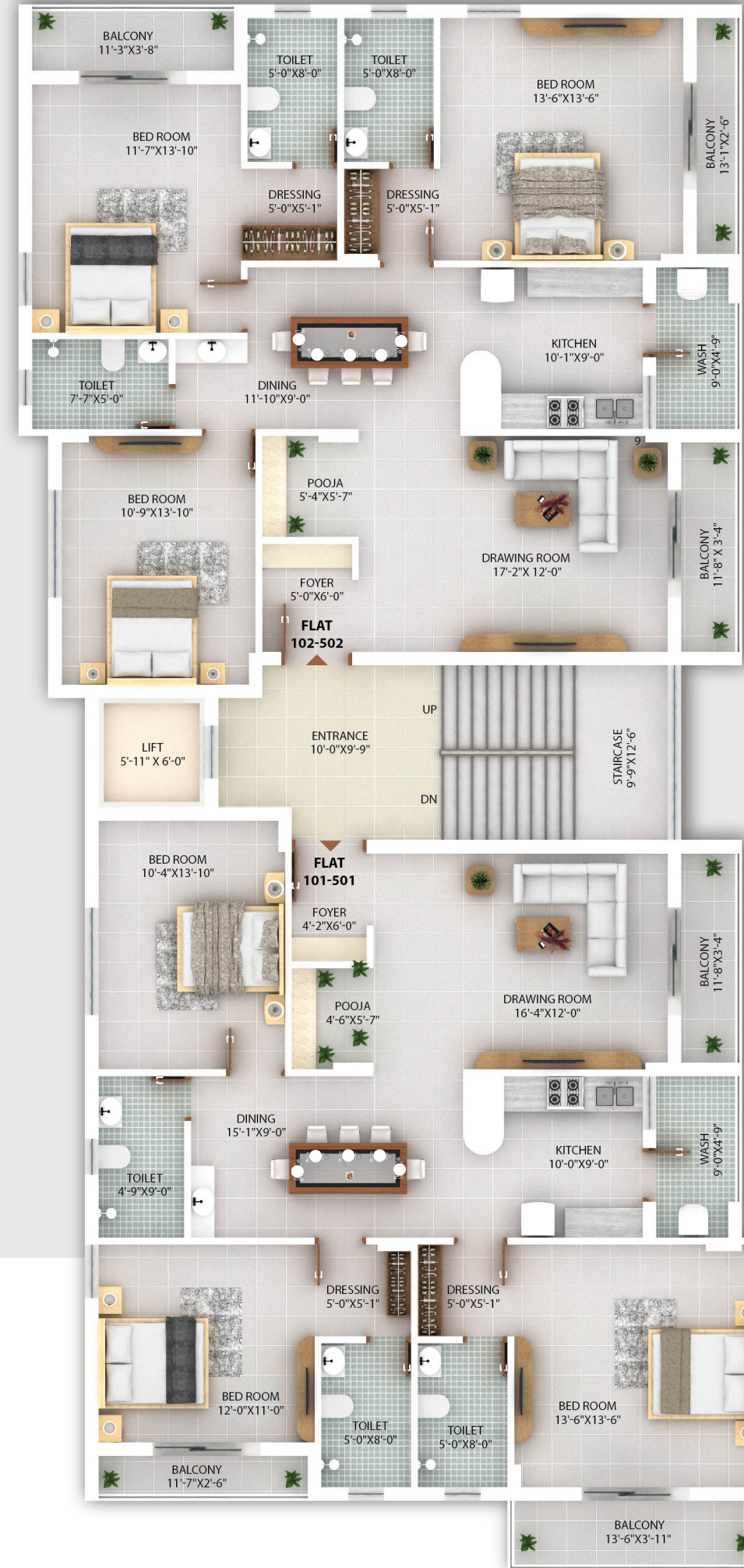
BLOCK - B TYPICAL 1ST TO 5TH FLOOR
