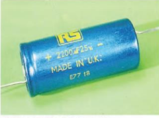
(b) Aluminium electrolytic capacitor
