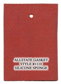
**Features:** Resilient, stable into high temperatures - very inert. Good resistance to sunlight and ozone degradation.
