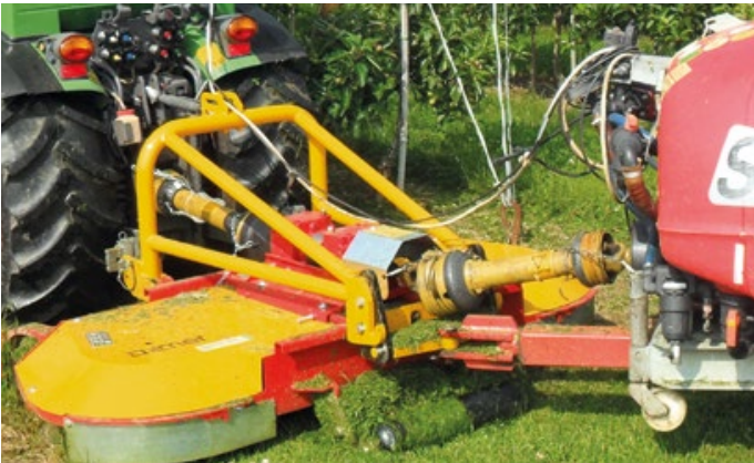
Mulch-spray combination The special frame optimally transfers the load of the trailer drawbar to the tractor, while the rotary mower can move freely.
