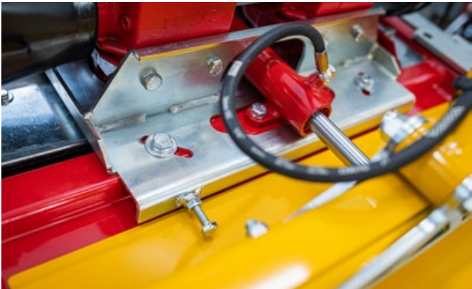
This is how maintenance is fun Simply incline the gear plate with two setting screws and the V-belts are retightened.
