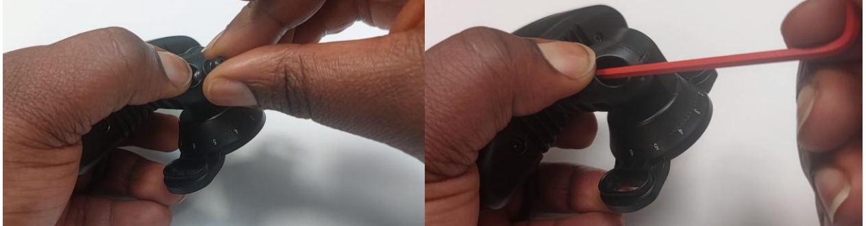
Figure 41: fixing the camera to the mounting bracket with the third hex head screw
