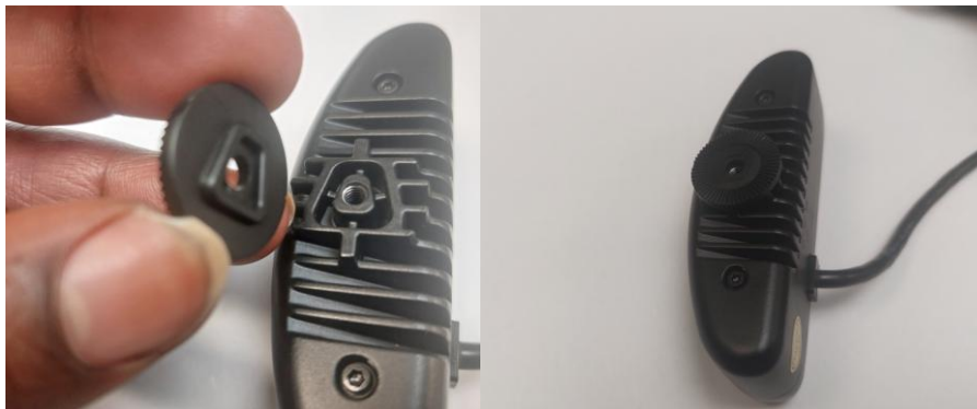
Figure 32: The fitting facing of the plastic face with the back of the camera
