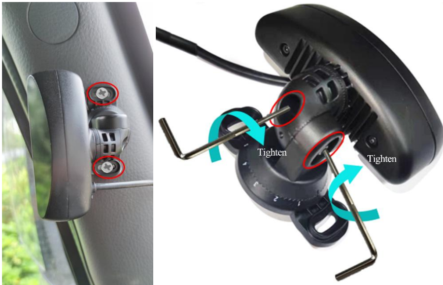
Figure 54: A-Pillar Driver facing camera showing self-tapping screw fixed on the lower section of the base of the bracket and the lens positioning hex head screws tightened.
