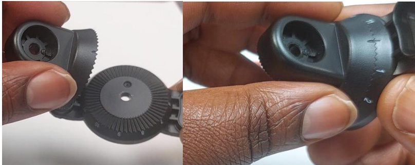
Figure 35: A-Pillar mounting bracket second and third pieces being fixed together.
