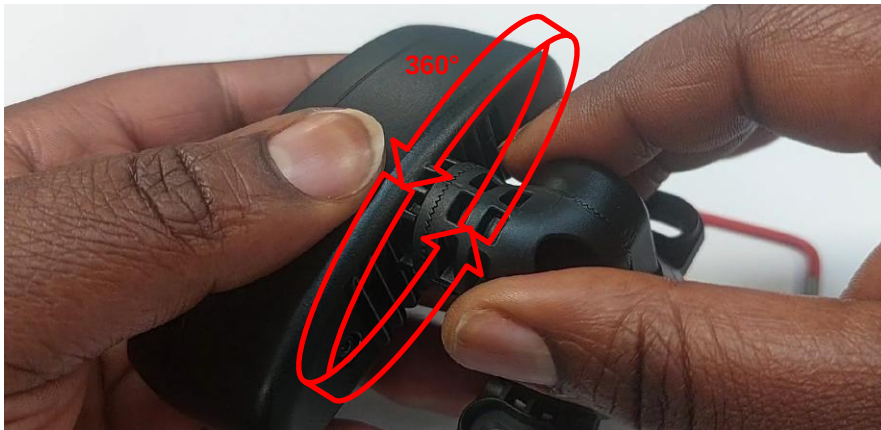
Figure 51: A-Pillar Driver facing camera showing the degree of movement of the camera head/top bracket piece joint when it hex head screw is loosened.
