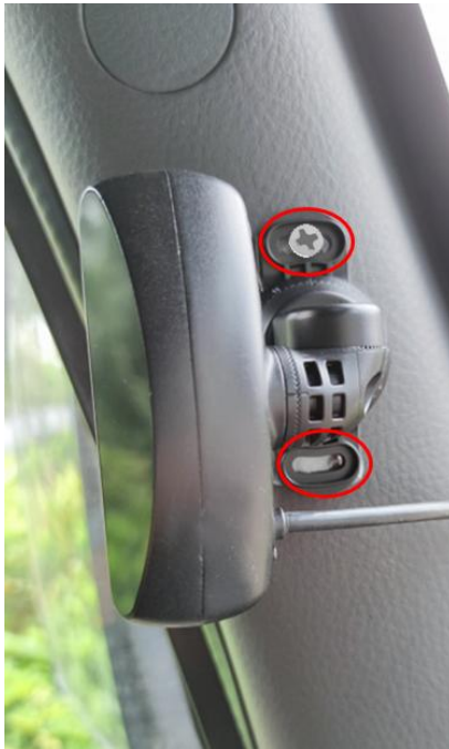
Figure 49: A-Pillar mounted DFC camera using only on self-tapping screw to hold the camera in place
