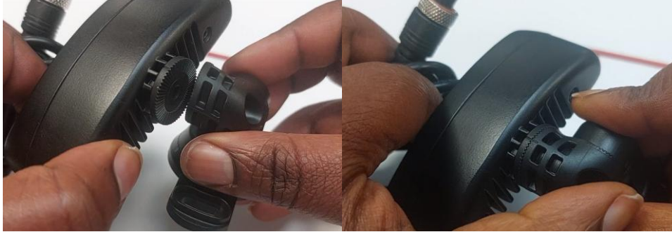
Figure 40: Fitting the camera to the mounting bracket
