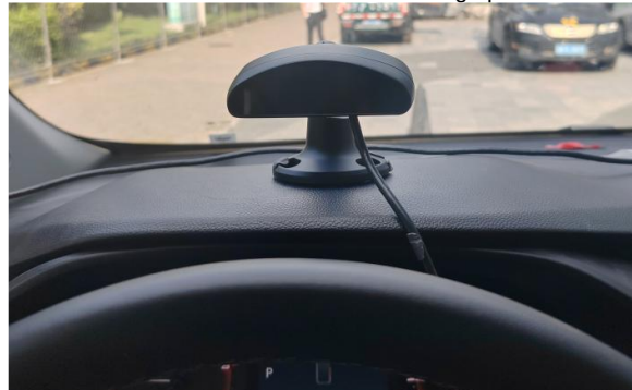
Figure 46: Dashboard Installation direction, the Camera is standing in the upright position.
