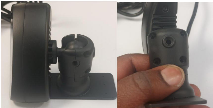
Figure 27: Fitting the second piece of the mounting bracket to cover the ball joint
