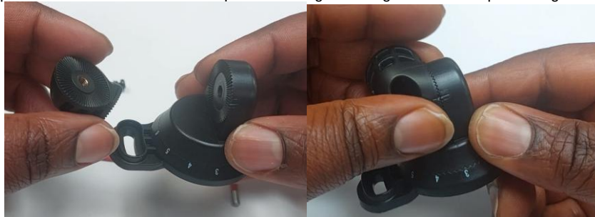
Figure 37: A-Pillar mounting bracket connecting the top to the middle piece of the bracket
