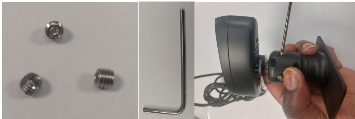
Figure 29: Fixing the orientation of the camera with the silver grub screws.
