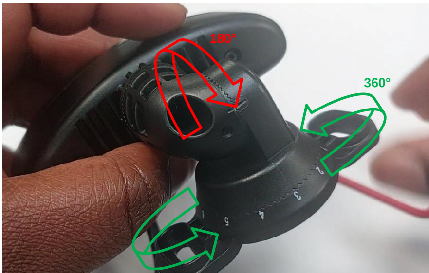
Figure 52: A-Pillar Driver Facing camera showing the degree of movement of the top piece and middle piece joint (red) and the Middle piece/base piece joint (green)
