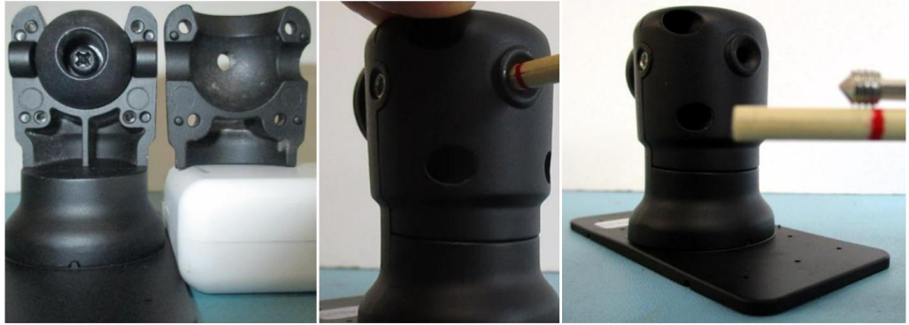
Figure 45: Pictures showing base of the ball joint at 90-degree angle, the hole at the base of the ball is about 16mm deep while the middle grub screw is only 5mm long.
