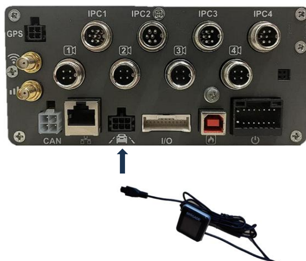
Figure 60 MDR-HWU-U connection diagram to MDR 644 direct connection
