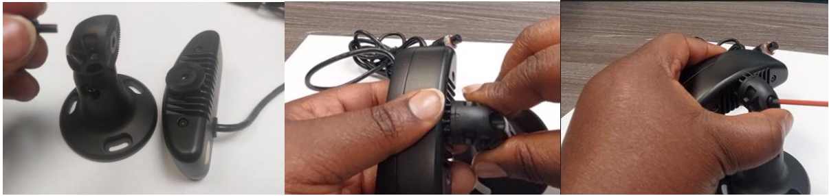
Figure 33: Fitting the camera to the mounting bracket
