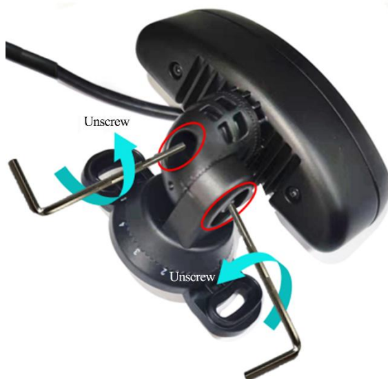
Figure 50: A-Pillar Driver Facing Camera showing the direction to turn the hex keys in order to unscrew the lens positioning hex head screws.
