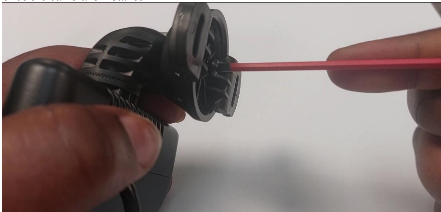
Figure 53: A-Pillar Mounted Driver facing camera showing the adjusting hex head screw at the base of the bracket
